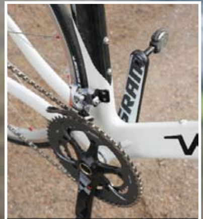
The PHX uses a SRAM Red groupset that allows for both rapid and exact shifting
